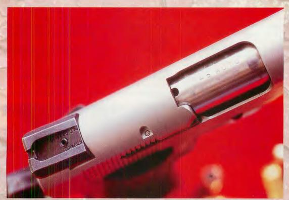
At the rear of the barrel's hood, is a cut to reveal the presence of a round in the chamber, if there is sufficient light to see it.
